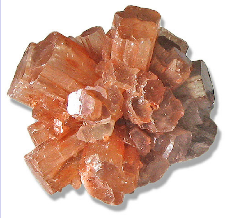
Aragonite - CaCO 3 Orthorhombic H = 3.5-4 S.G = 2.94 Cleavage: one plane
